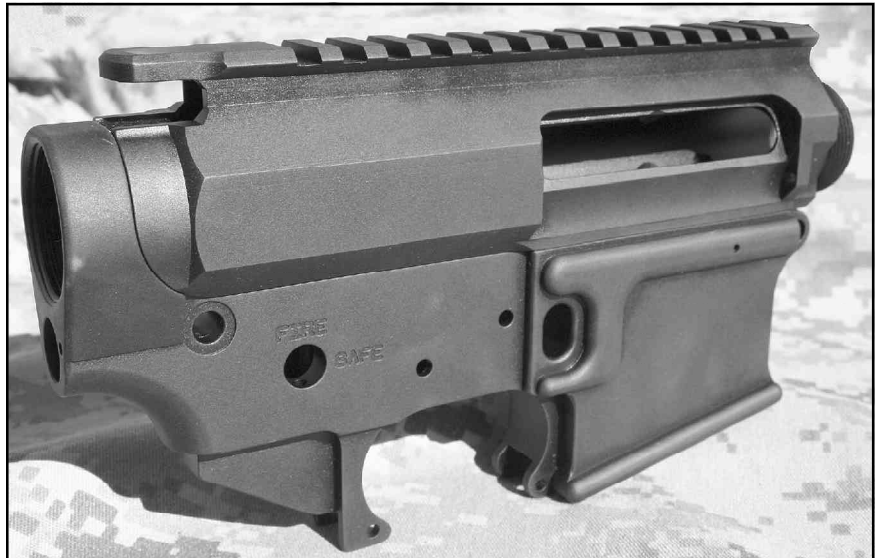
Above: Sun Devil second-generation upper receiver and lower receiver prior to assembly. The Upper is easy to identify because of its lack of forward assist and octagonal shape.
